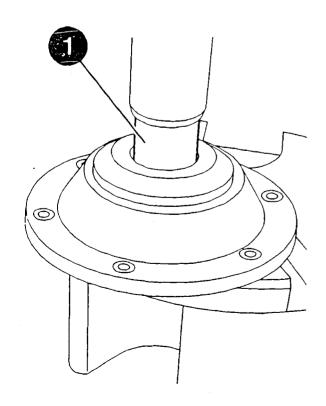
Installing cylindrical roller bearing in drive/reduction gear end shield
